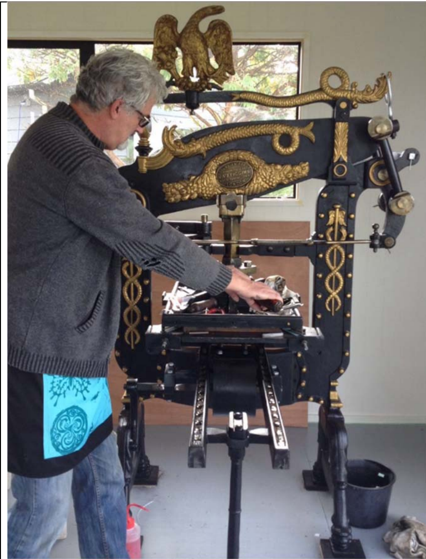
The Columbian Iron Hand Press manufactured by V&J Figgins of London in 1880 here at the studio in Helensville.
